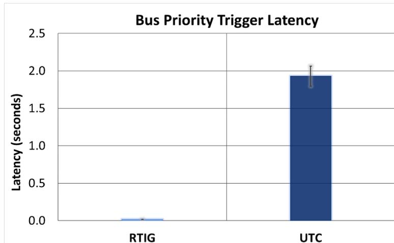
Providing bus priority locally still requires a method of communicating with the Data Relay Unit that handles the RTIG feed from the bus operators but the reduction in latency reinstates the local priority level of service that was previously lost.
